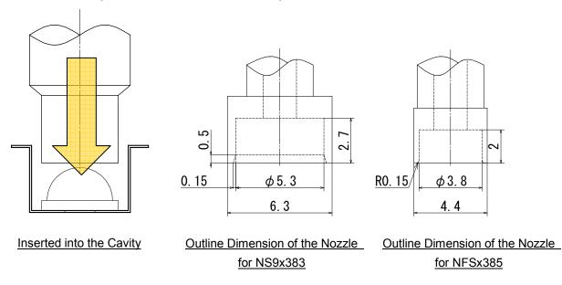
The pick-and-place nozzle is chamfered so as to form a "C Surface" (a sloped surface) and an "R Surface" (a curved surface), enabling a smooth mounting of the LEDs. Such design of the nozzle can prevent the LEDs from tilting in the cavities.
