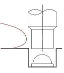
The nozzle can appropriately pick and place the LED.
